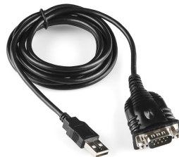
Figure 11.1: RS-232 to USB adaptor
